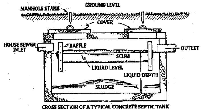
A septic tank allows heavier solids to settle and be partially decomposed by bacteria to form sludge.
